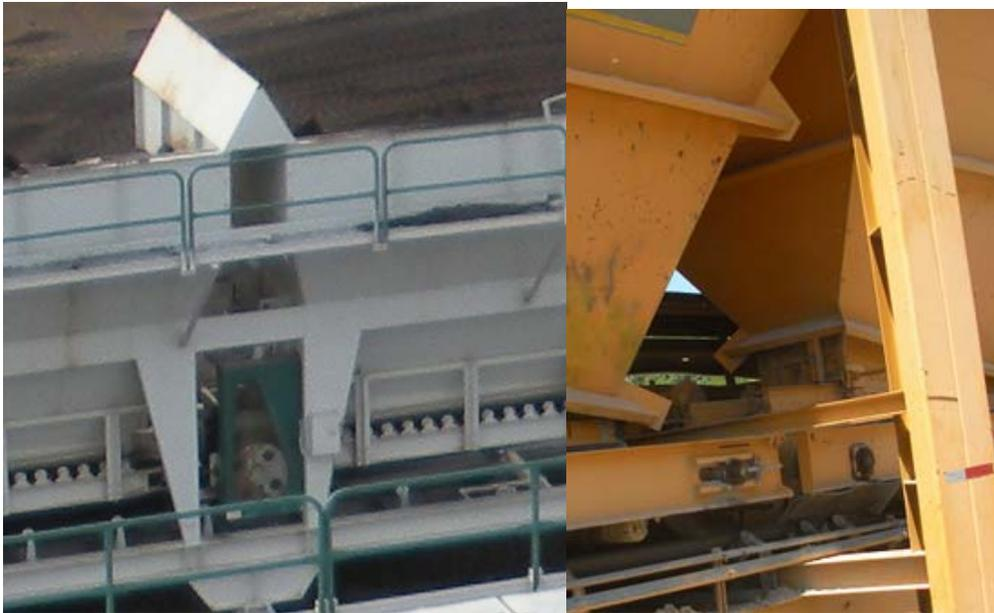
Taking the confinement issue one step further, many existing rap bins have bin support structure and Bin Feeder Conveyor Drive Pulley-Sprocket arrangement on one side of the bin and the Loader Ramp barricading the other access to the confined space. In some cases, the task looks impossible unless one was to assemble the scale inside the confined space.
