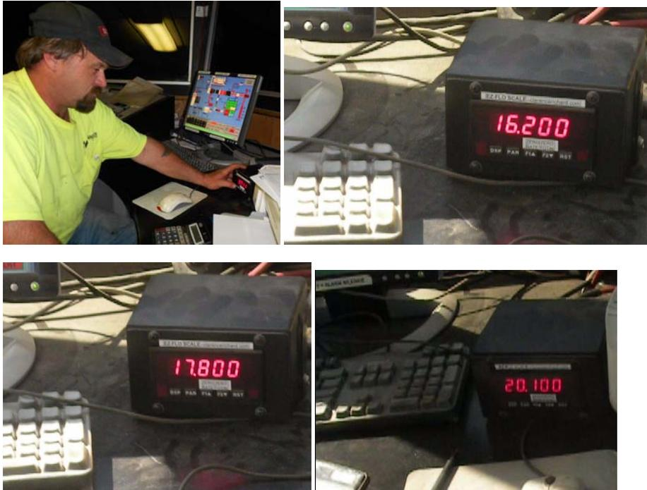
Henningsen Plant Manager Duane Updike shown here observing the Bin Flow Rate changing from plus or minus 15% while the feeder speed is running at a constant speed. The same 15% deviation was observed at flow rates as low as 6.75 TPH to 25 TPH. These sequential pictures illustrate the rate changes with the gate setting at 4" and the 21% feeder speed. The third picture illustrates, by the changing shadows on the key, it was some time later that a major plus deviation was happening.
