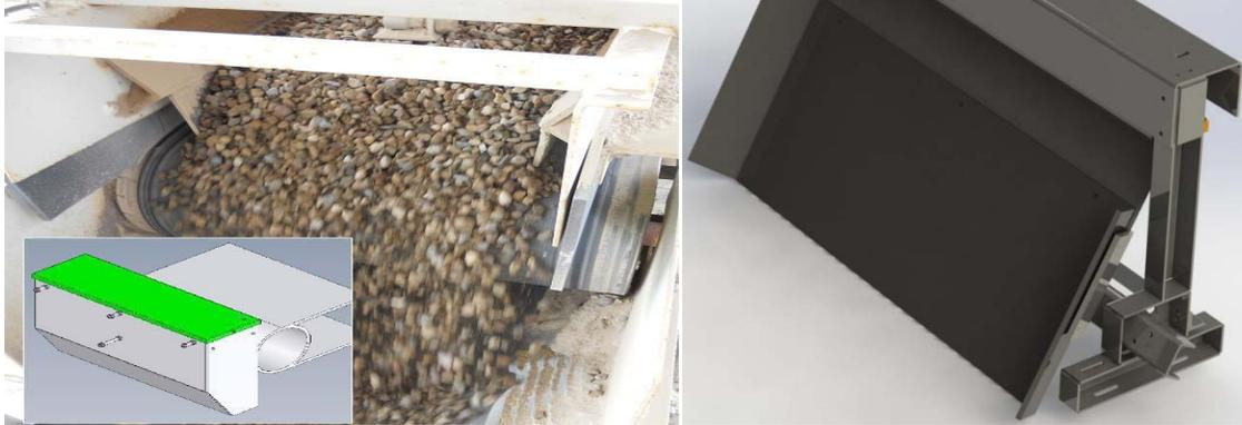
Taking this all into consideration, it was decided to minimize the size as much as possible, design it to be assembled inside or outside of the confined area, easily change from wide feeder belts to narrower one and mounted on skids with slots to slide the scale out of the flow when using the bin for RAP but keep it in the flow for FRAP (Fine RAP). FRAP has 8% oil and is worth close control and does not usually have big chunks.
