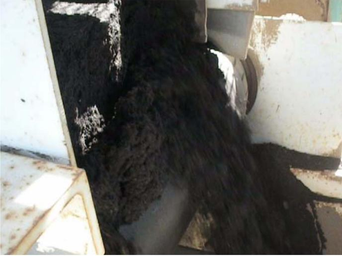
The job was difficult. Generally, the area is confining. The distance between the RAS Feeder Head Pulley and RAP tail pulley and both of their support structures are 20 " and the distance between the bottom of the Feeder Belt and the center of Collector Belt was 12", not to mention the troughing rollers using up that 12" space. Then consider the Material entering Fins overhanging the head pulley by a foot.
