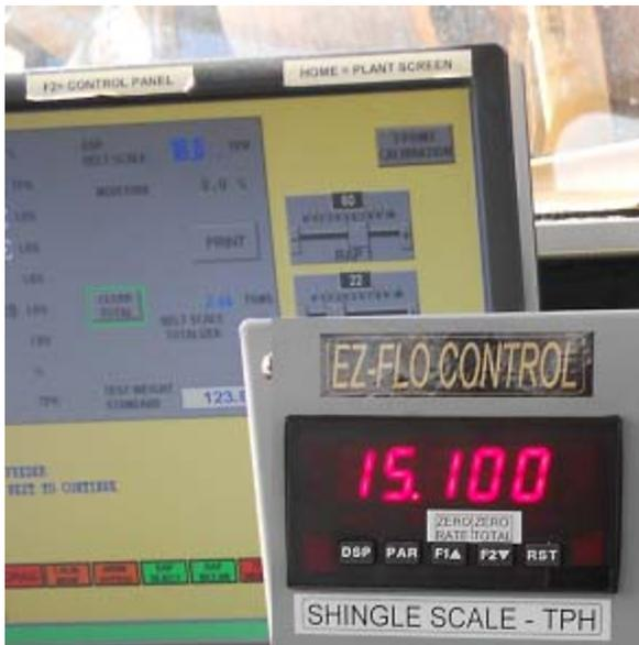
The Impact Scale is reading in real time is normally being monitored by the plant computer. Plant computers are programmed to either compensate for the oil when the Rap Scale deviates from Set point or to increase or decrease both Feeder Bin Speeds. Either way, one scale is not enough.
