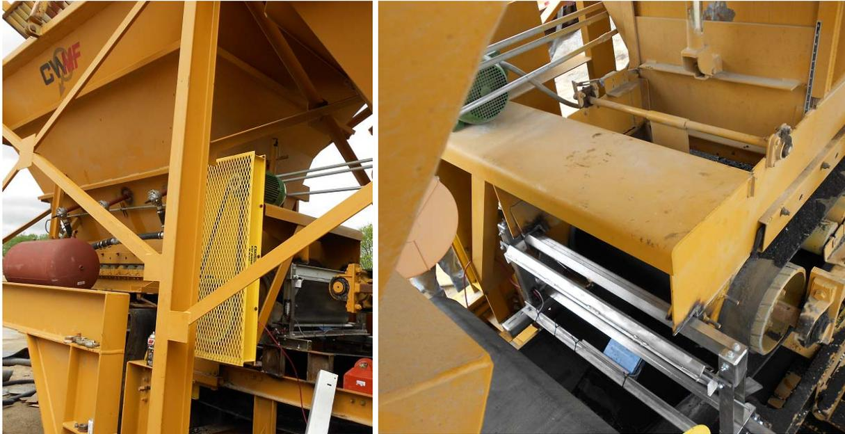
The Flow Scale impact plate is mounted 6" away from the end of the Belt Feeder Head Pulley.
